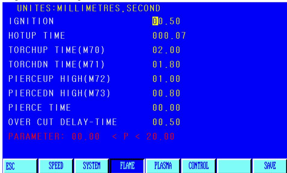
Ignition delay---flame cutting, when performing M20, open the high voltage ignition switch delay time.
