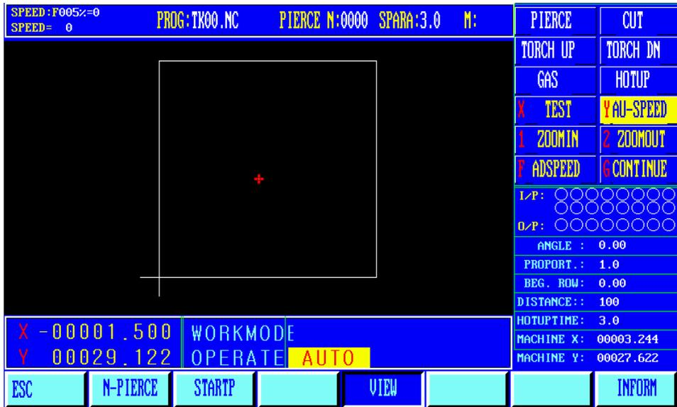
Select this function, the system display graphics processing procedure, and marking punch points are numbered sequentially, graphics origin points have cross cursor. Press [1] 1 time magnification graphics (up to three times, enlarge 8 times), press [2] graphics recovery, according to the **【↑】【↓】【←】【→】** key mobile graphics display position.
