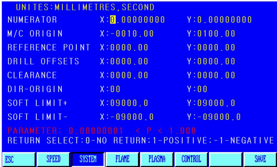
Pulse equivalent - electronic gear molecules and the ratio of the denominator is the pulse equivalent, unit microns, converted to X 1000 MM.
